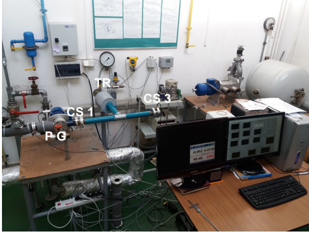
Figure 1: General view of the experimental test stand. P-G – pulse generator, CS 1,2 cross section 1,2, TR – tube resonator.
